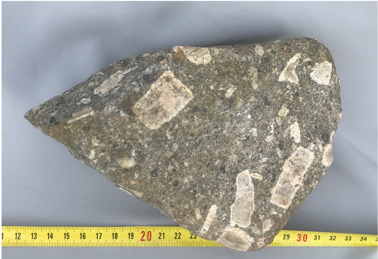
Fig. 13 : Not-bleached surface, showing the rectangular pieces of the crinoidé stem
