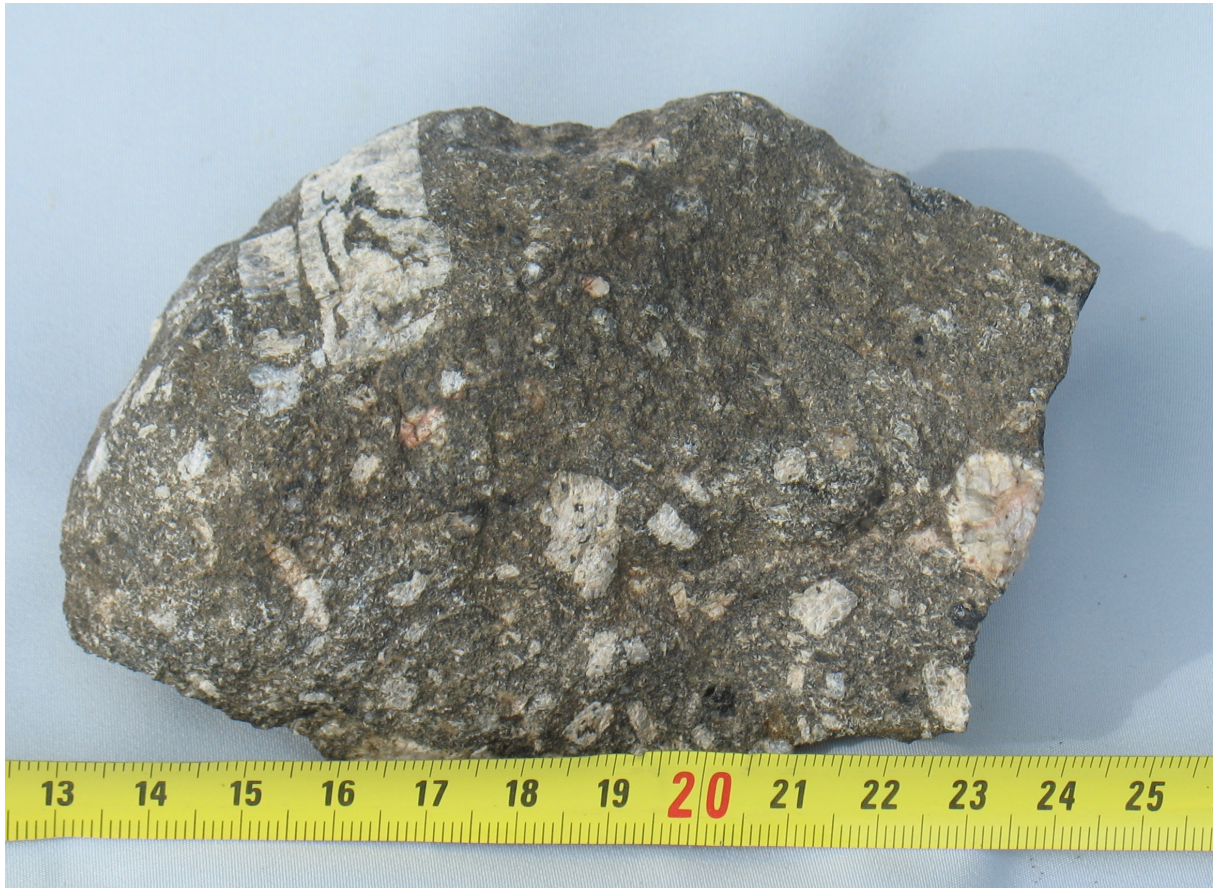
Fig, 14 : Fresh sample of the sedimentary rock of Fig. 11 and 12. Here the hornblende is seen. (IMG_3331.jpg) Thickness of sample: 4 cm.
