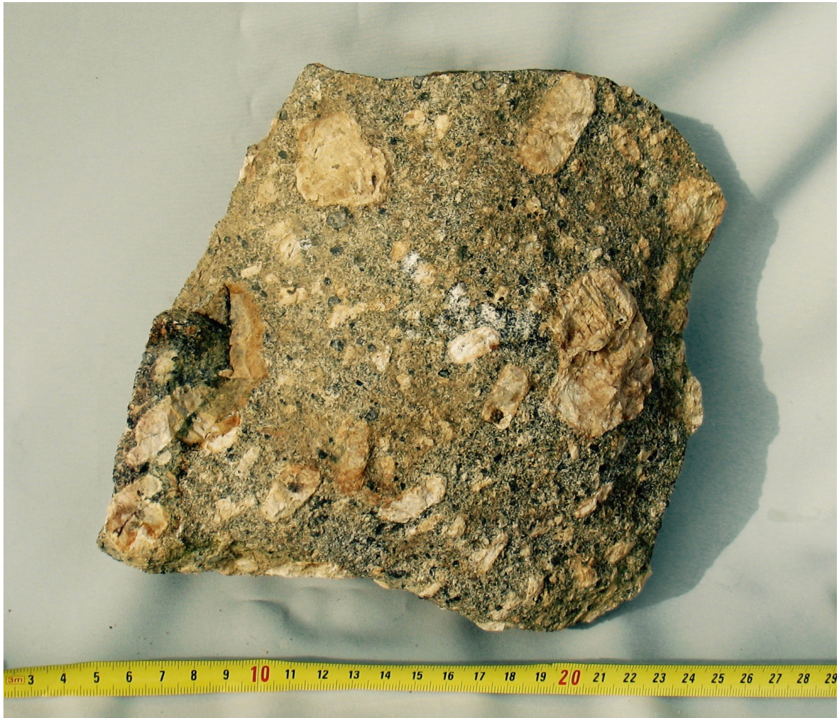
Fig. 12 : Rear side of Fig. 11. Thickness of sample ca 10 cm. Note the quadratic hornblende crystals. (IMG_3330.jpg)
